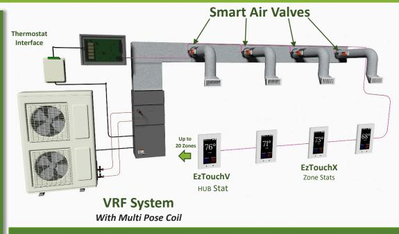
Reduce long refrigerant runs & equipment costs by replacing indoor units with Smart Air Valves (SAV)
