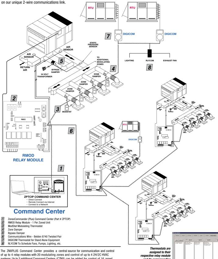
systems. Up to 3 additional Command Centers (CZNX) can be added for control of 16 zoned units and 80 thermostats or devices. The Command Center stores system information and scheduling in its non-volatile memory.
