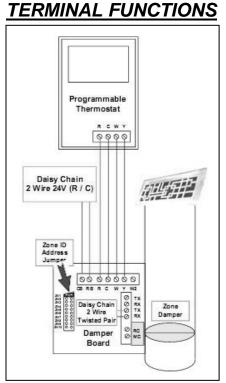
RC- 24vac input to damper motor MC- 24vac common input to damper motor
