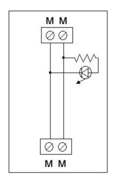
MM- 24 VAC input to damper motor
