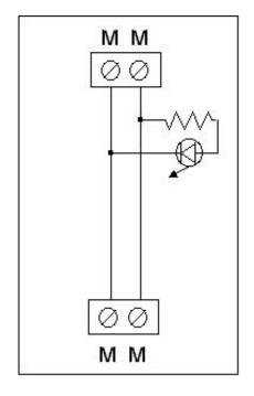
MM- 24vac input to damper motor. Power open.
