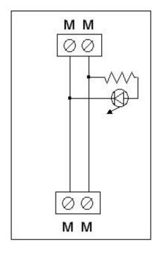
MM- 24 VAC input to damper motor. Power open. MM- 24 VAC output to damper motor
