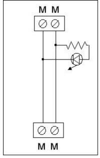
MM- 24 VAC input to damper motor MM- 24 VAC common input to damper motor
