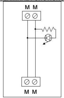
MM- 24vac input to damper motor MM- 24vac common input to damper motor
