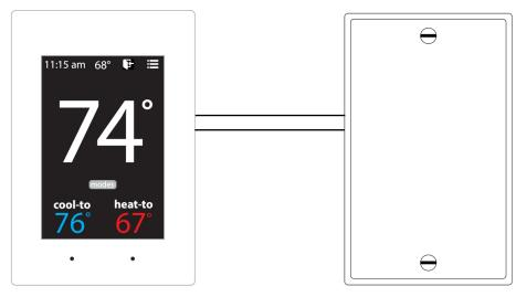
Use 18 gauge copper wire to connect the thermostat to the remote sensor. Max length up to 200'.
