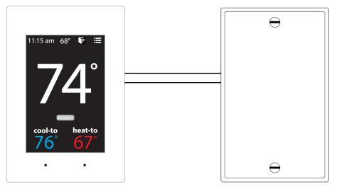
Use 18 gauge copper wire to connect the thermostat to the remote sensor. Max length up to 200'.
