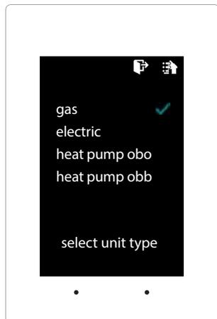
The SATouch is designed as a universal GAS/ELECTRIC/HEAT PUMP thermostat. Factory default is set for GAS operations.
