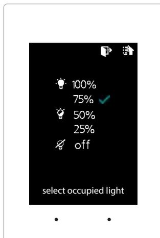
The brightness of the thermostat during occupied mode is adjustable from 100% down to off.
