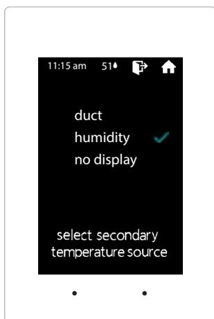
*The thermostat can display the supply air duct, relative humidity, or no value will be displayed at the top of the home screen. An optional LAT temperature sensor must be installed to report outside air or supply air duct temperature.*
