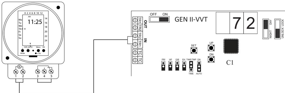
5. The Normally Open switch contacts on the time clock 3 and 5 are wired to the TC terminals on the GEN II Controller. See wiring diagram below.
