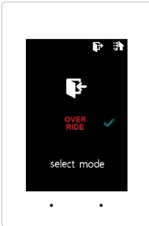
When a thermostat displays "unoccupied mode" , a 2-hour temporary override maybe initiated.
