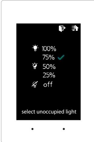
The brightness of the thermostat during unoccupied mode is adjustable from 100% down to off.
