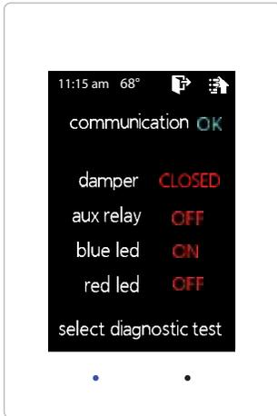
The EzTouch Diagnostic screen will allow you to confirm communication with the GEN II controller and allow you to confirm damper, aux relay, and LED operation.
