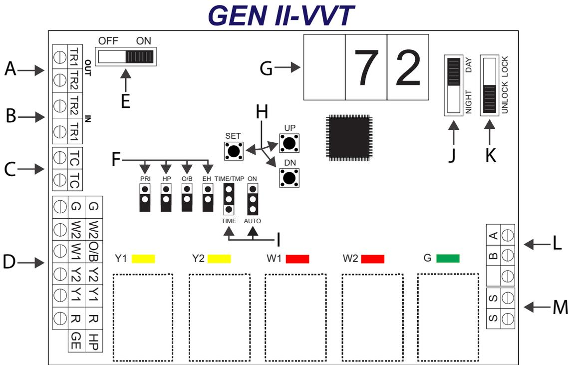
The *GEN II* is equipped with a **Digital Display (G)** that constantly displays **Leaving Air Temperature from the unit**. The display and 3 buttons beneath the display provide the installing contractor the ability to tailor the system to your specific application.
