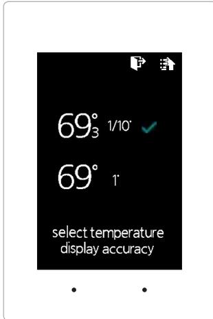
*Display accuracy allows the thermostat to display the room temperature in 1/10° or 1°.*
