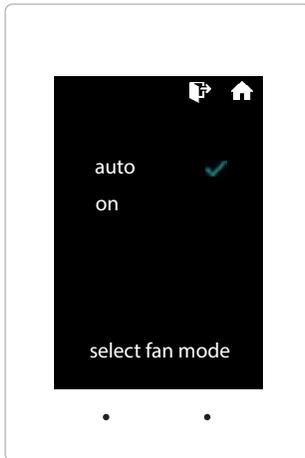
Fan operation is configured for either Fan ON or AUTO. When system is configured for ON operation, the Fan will run during Occupied schedule and will revert to Auto operations during Unoccupied schedule. When thermostat is configured for Auto operation, Fan will only run when there is a call for heating or cooling.
