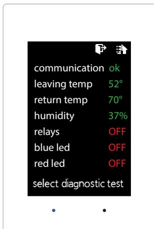
The SATouch Diagnostic screen will allow you to confirm communication with the GEN II controller and allow you to confirm the relays operation, LED operation and report the leaving/return temperatures as well as the relative humidity.
