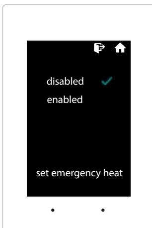
The SATouch has an emergency heat function that will lock out the compressor, and energize the Aux heat in the unit.
