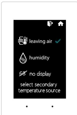
Temp source allows the thermostat to display the leaving air temperature or the relative humidity at the top on the home screen. A LAT sensor needs to be installed to report this reading. It will read 00 if no sensor is installed.
