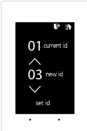
Every thermostat in the system needs a unique ID. They must be ID'ed in numerical order the way the communication wire is daisy chained. No duplicate addresses.
