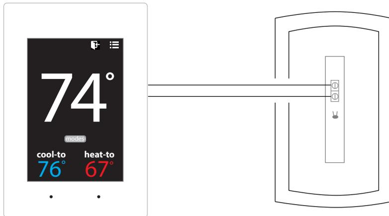
Install thermostat per installation instructions. All remote sensors include a wiring harness. Plug wiring harness into the back of the thermostat, this will provide two wires to connect the remote sensor to the thermostat. Per the drawing above, wire the remote sensor in parallel, one wire from the thermostat will connect to + terminal on the sensor, the second wire will connect to - terminal using 18AWG thermostat wire. Verify sensor operations.
