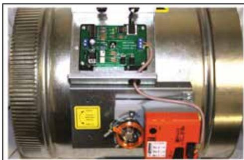
1. Locate the Integrated Pressure Control (IPC) and air tube on the bypass damper. Drill hole into the side of the supply duct 2' after the bypass and before the 1st supply take-off.
