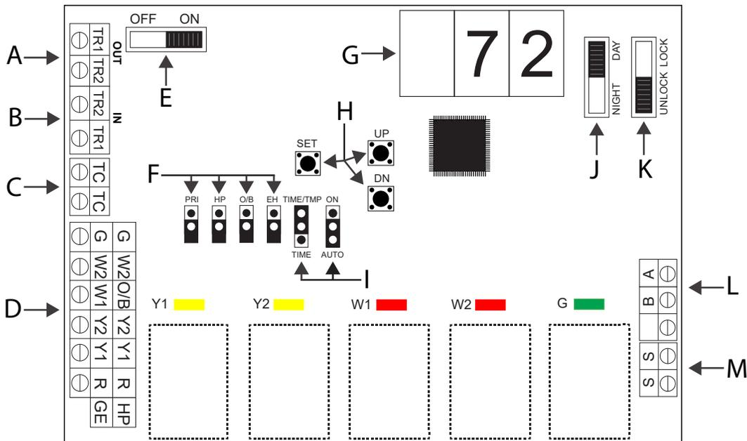
The **GEN II** is equipped with a **Digital Display (G)** that constantly displays **Leaving Air Temperature from the unit**. At startup, this display also reports the number of thermostats communicating with the **GEN II** controller. The display and 3 buttons (**H**) beneath the display provide the installing contractor the ability to tailor the system to your specific application.
