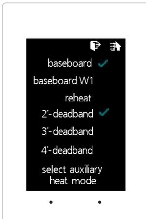
The zone thermostat provides the following Auxiliary Heat options; Baseboard, Baseboard W1 and Reheat with configurable dead band of 2°, 3°, or 4°.
