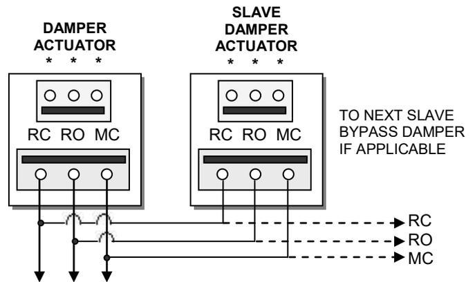
To Static Pressure Control, as shown on the Bypass Wiring Diagram on the next page.
