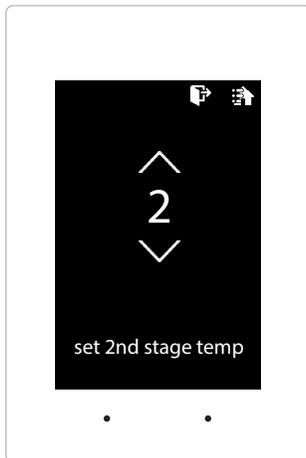
The SATouch's 2nd stage operation is based on room temperature. Staging is adjustable from 2°- 8° from thermostat room temperature.
