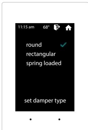
*The EzTouch needs to be configured for the type of damper that it is wired to. There are 3 options, round, rectangular or spring loaded.*
