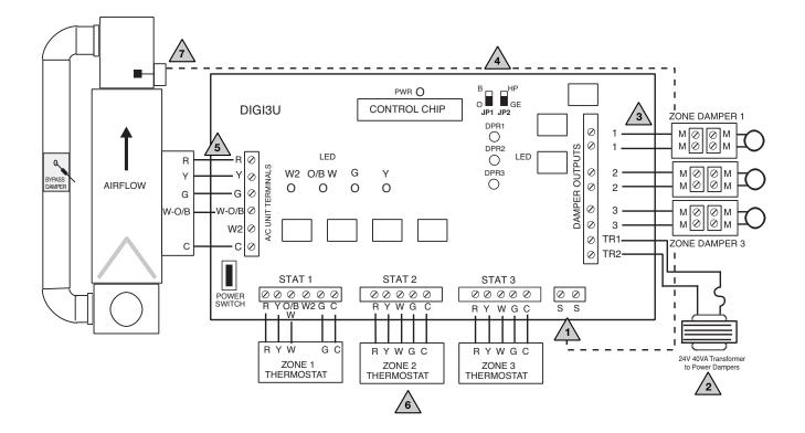
S S – terminals for LAT capacity control. If not applied, leave 1k ohm resistor in place; and field supplied high and low limits should be added.
