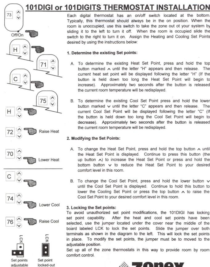
Each digital thermostat has an on/off switch located at the bottom. Typically, this thermostat should always be in the on position. When the room is unoccupied, use this switch to take the zone out ot your system by sliding it to the left to turn it off. When the room is occupied slide the switch to the right to turn it on. Assign the Heating and Cooling Set Points desired by using the instructions below:
